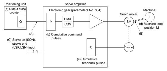
When a position shift occurs, check (a) output pulse counter, (b) cumulative command pulse display, (c) cumulative feedback pulse display, and (d) machine stop position in the above diagram.
